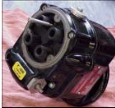
Slick magneto with timing pin inserted
