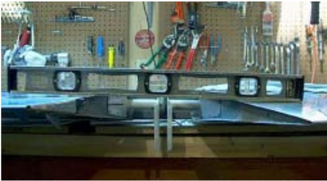
that swing parallel to the outboard edge of the horizontal stabilizer are clamped flush to the HS. When I did that, as you can see, there was about a 3/8" drop from the left elevator to the right one.
